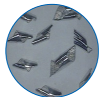
Chip Breaker End mill Chip Geometry
